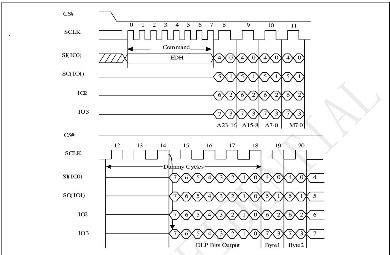
Note: 1. The DLP bit is also valid for 4-byte EDH and EEH instruction and QPI 4IO DTR read instruction.
