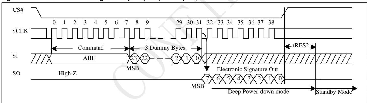
**Figure 9-50a Read Electronic Signature (RES) Sequence (QPI)**
