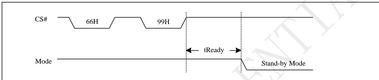
**Figure 9-64a Software Reset Sequence (SPI)**
