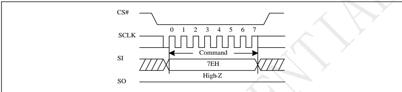
**Figure 9-62a Global Block Lock (QPI)**
