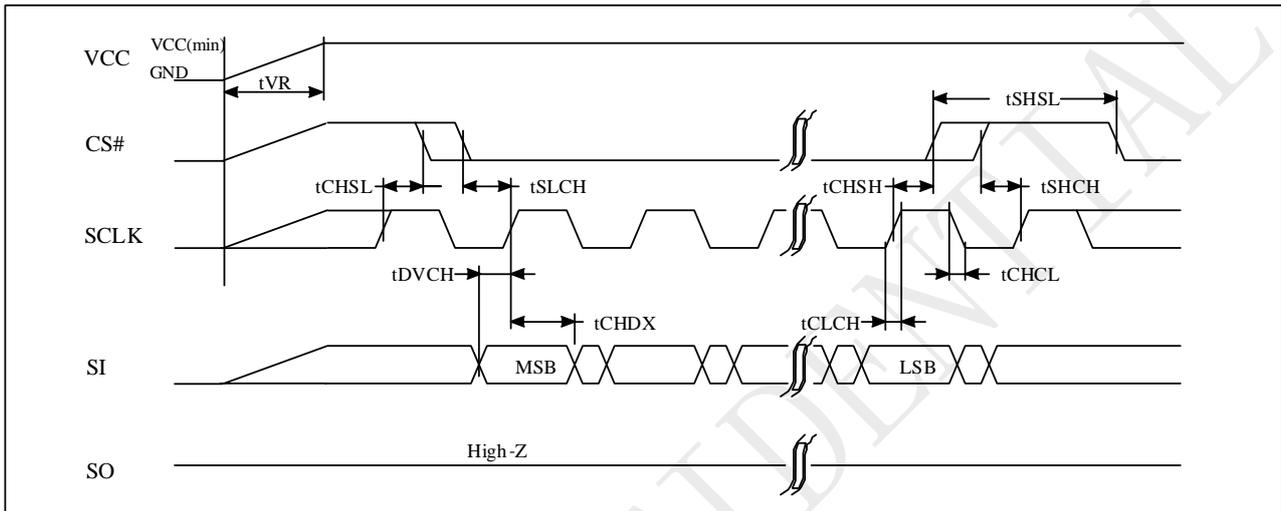
Figure 5-9 Power-up Timing
