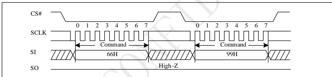
**Figure 9-64b Software Reset Sequence (QPI)**
