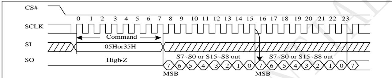
Figure 9-5a Read Status Register (RDSR) Sequence (QPI)
