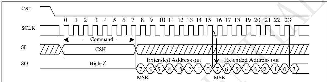
**Figure 9-9a Read Extended Address Register Sequence (QPI)**
