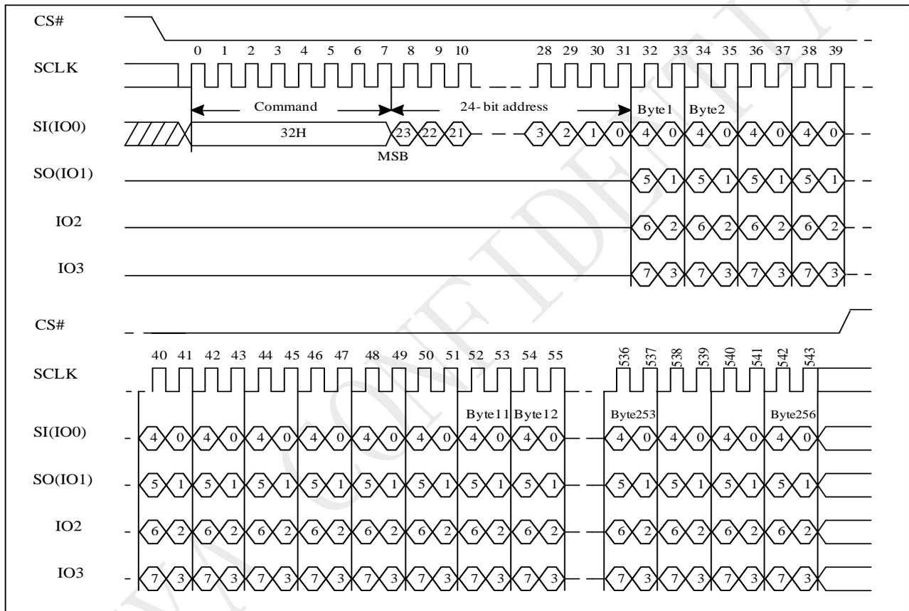
Note: 32-bit address is required when the device is operation in 4-Byte Address Mode.
