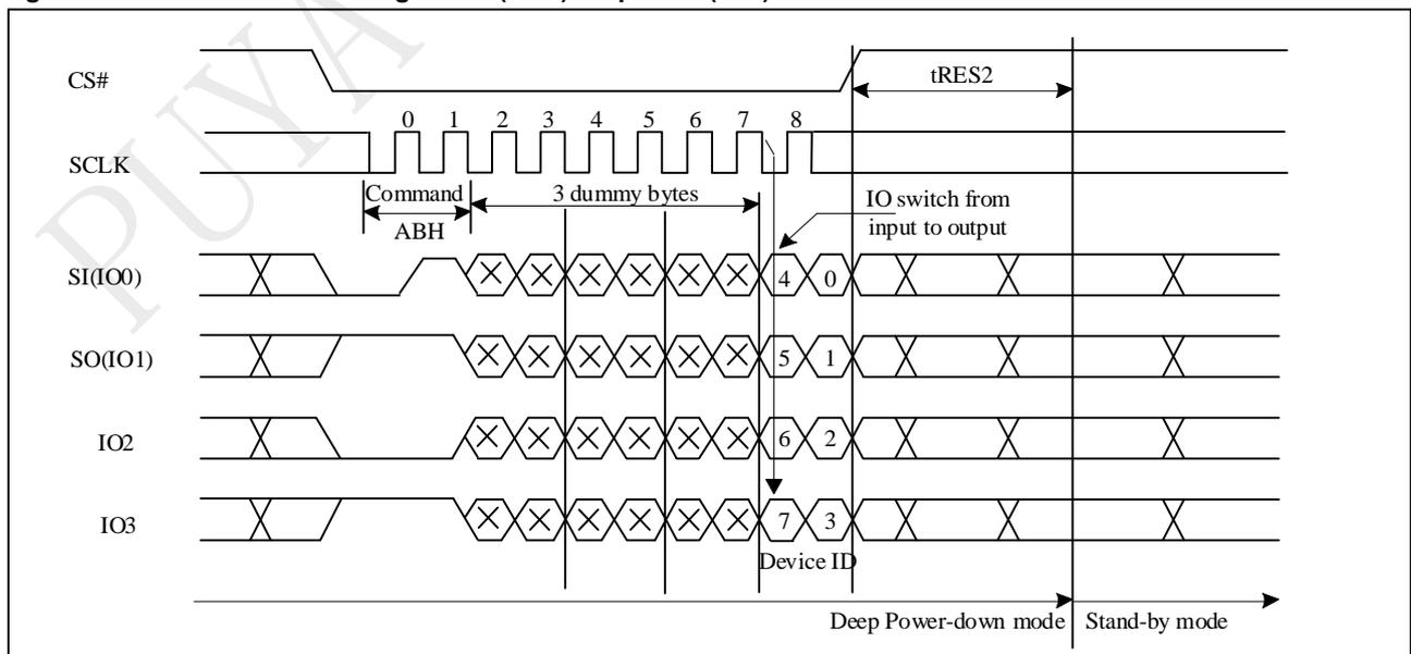
**Figure 9-50b Release from Deep Power-down (RDP) Sequence (SPI)**
