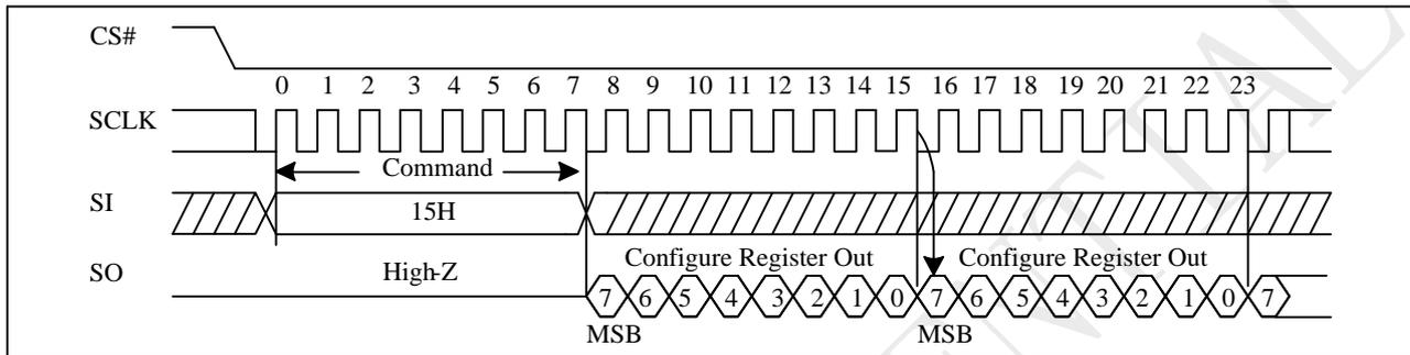
**Figure 9-6a Read Status Register (RDCR) Sequence (QPI)**
