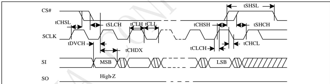
Figure 5-5 Output Timing
