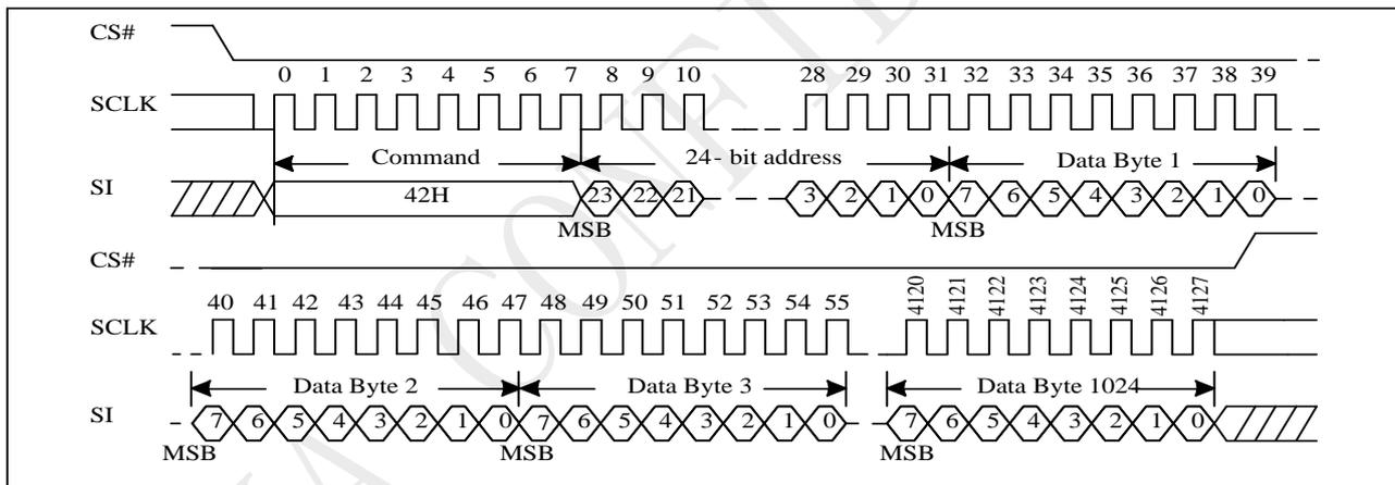
Figure 9-47a Program Security Registers (PRSCUR) Sequence (QPI)
