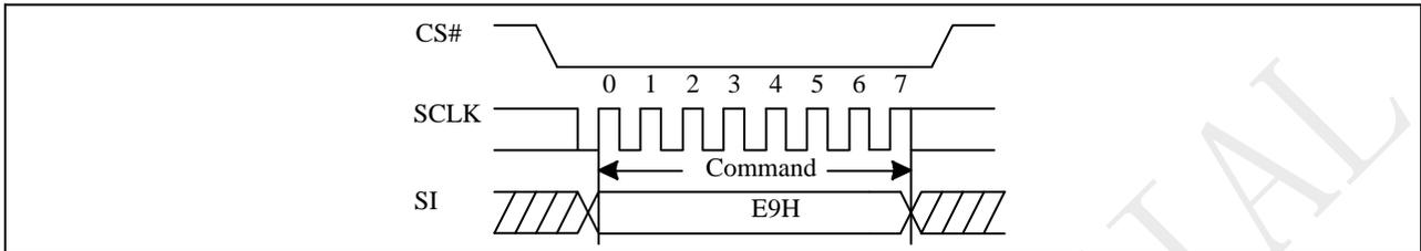
**Figure 9-12a Exit 4-Byte Address Mode Sequence (QPI)**
