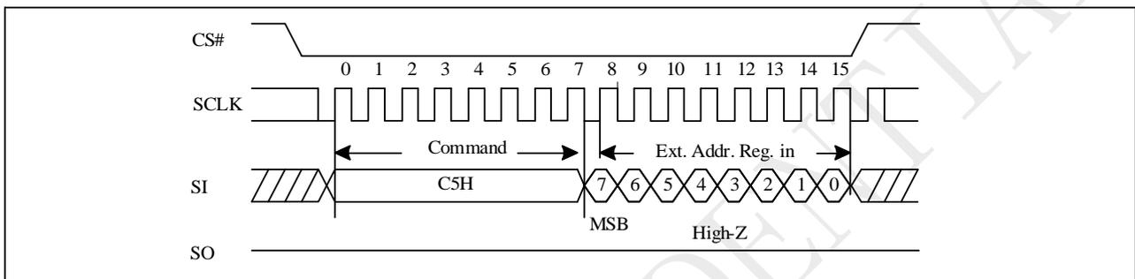
**Figure 9-10a Write Extended Address Register Sequence (QPI)**
