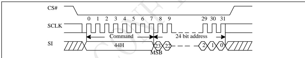
Figure 9-46a Erase Security Registers (ERSCUR) Sequence (QPI)
